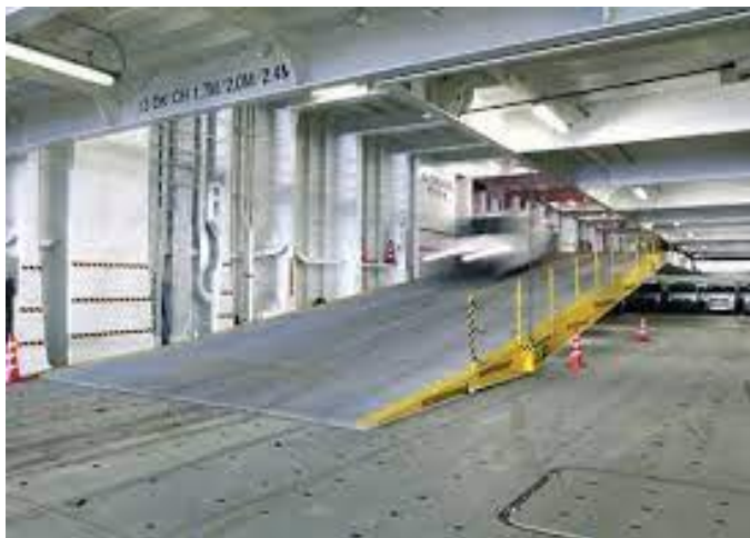
Figure 1: This is an example of the road that is used in the Ro-Ro to move the vehicles into the vessel. As we can see there is no any device or structure to slow car down while going into the vessel.
