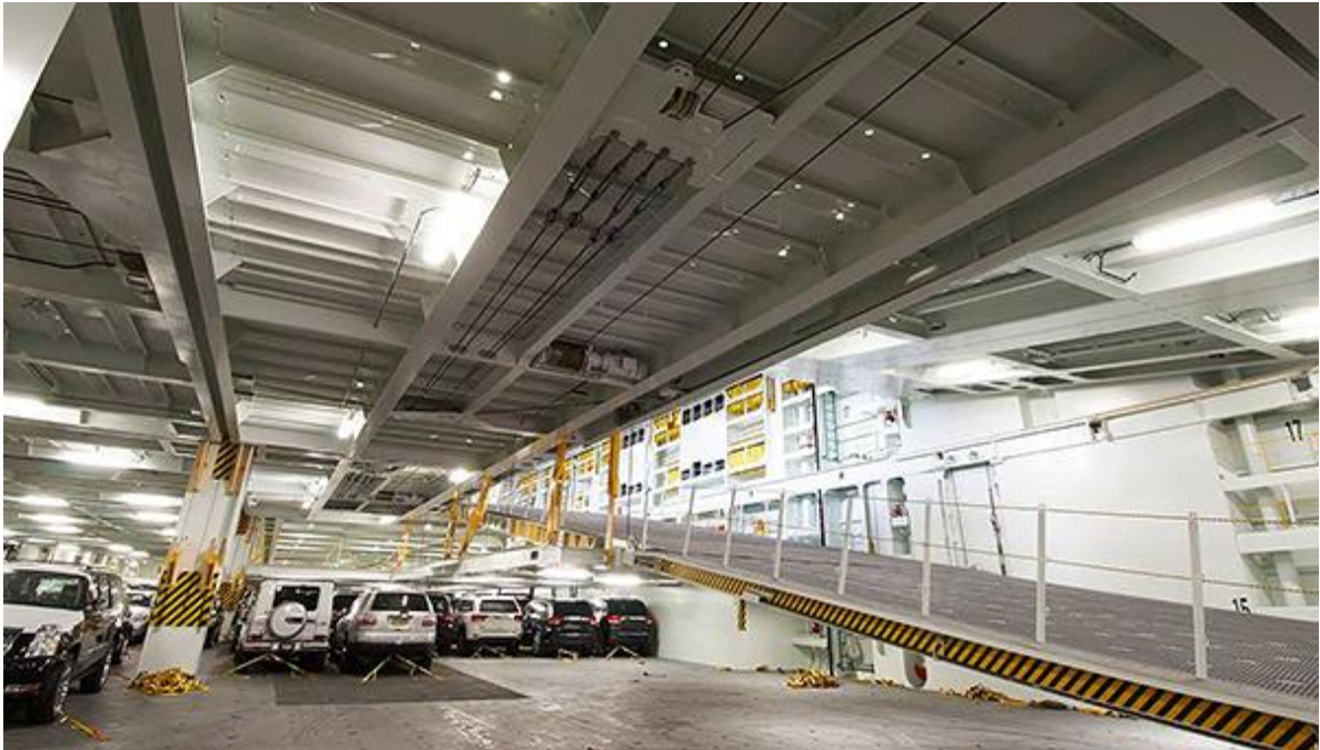
Figure 2: This is the layout inside of the RoRo as we can see there is no any extra object to hold the vehicle. If the strap snap due to rough weather it can damaged other vehicle and vessel.
