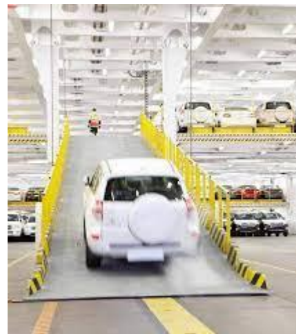
Figure 1: This is an example of the road that is used in the Ro-Ro to move the vehicles into the vessel. As we can see there is no any device or structure to slow car down while going into the vessel.
