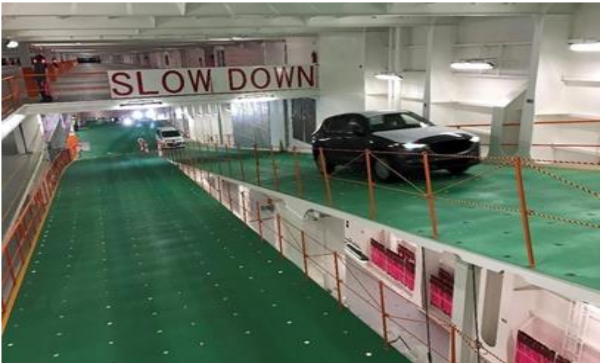
Figure 3: This is not a safe procedure going up the ramp since collision may occur if a brake failure happens. Hence why having a smart hump is important because it can hold the car from going backwards and colliding with other vehicle.
